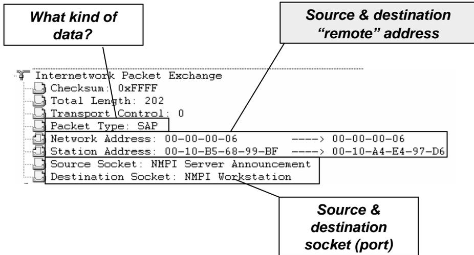
The IPX header contains fields that control the remote delivery of the packet.
